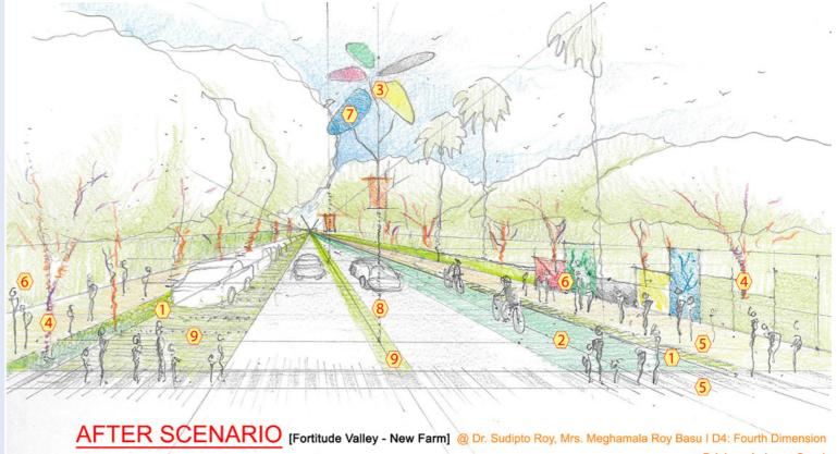
Ireplacing raised kerb with flush kerb to achieve one seamless continuous profile with different surface treatments for road, median, shoulder and sidewalk - thereby promoting universal access and inclusion, including provisions for elderly, disabled and visually impaired citizens Connected:
