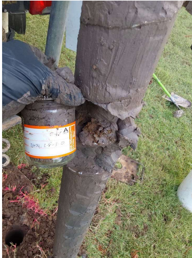
Photo 11: BH04 natural alluvial silty clay soil, with brown and orange organic matter from 2.2 to 4 m BGL.
