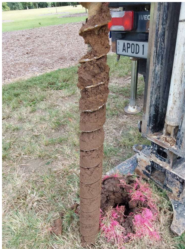
Photo 5: BH02 fill - reworked local soil from surface to 0.3 m BGL then natural silty clay to 1m BGL.
