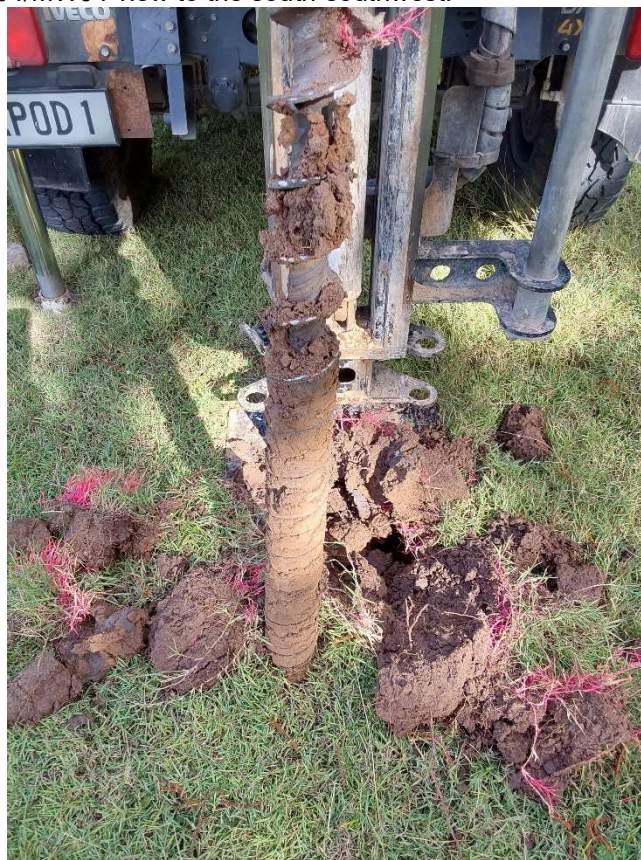
Photo 10: BH04 natural silty clay soil from surface to 1 m BGL.
