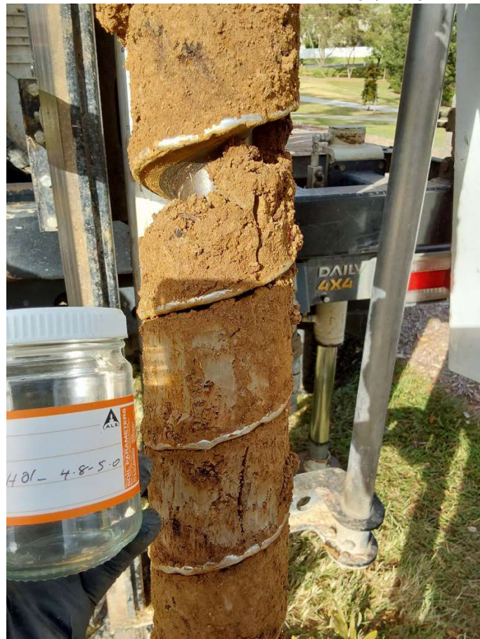
Photo 2: BH01 from 0.2 to 6.2 m BGL natural silty clay soil with trace sandstone inclusions.
