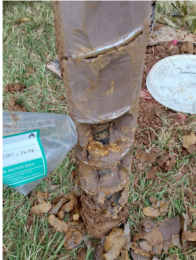
Photo 3: BH01 natural clay soils from 6.2 to 8 m BGL with yellow (jarosite) & orange mottle.
