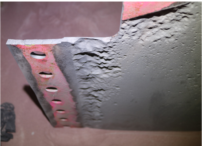
3-Way plate corrosion and pitting
