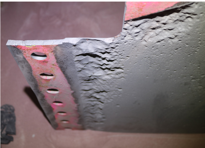
3-Way plate corrosion and pitting
