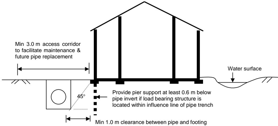
Case 2: Slab on ground structures built over stormwater pipe
