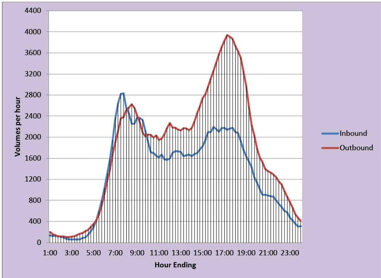
Figure 1 – Hourly Volume Profile at Lytton Rd / Latrobe St intersection
