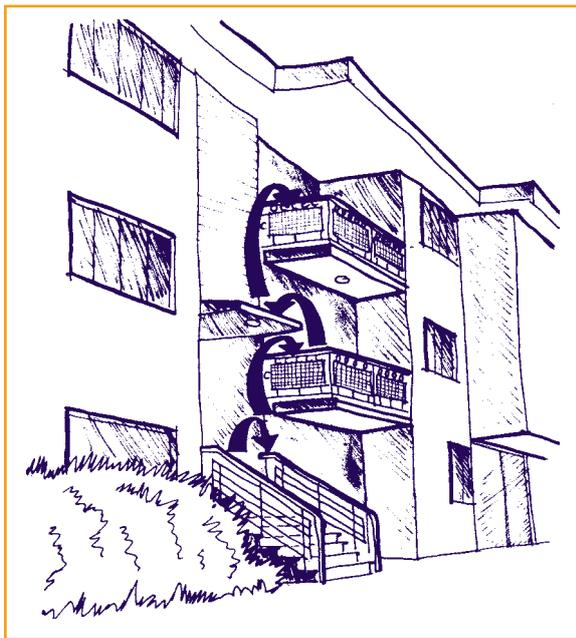
Figure j Building design should minimise features which create natural ladders
