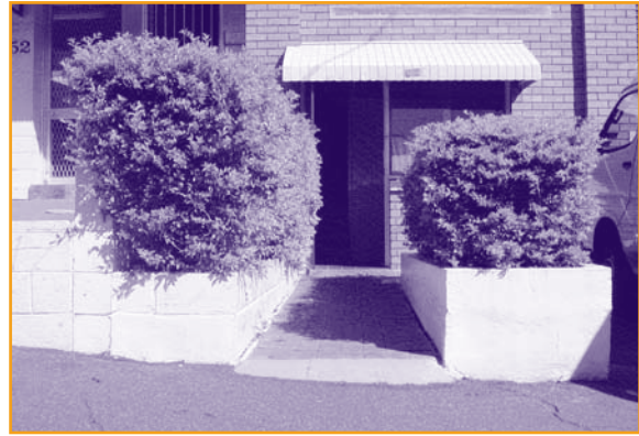
Figure k Retaining walls and vegetation obscure the entrance, providing a concealment point and a possible entrapment location.
