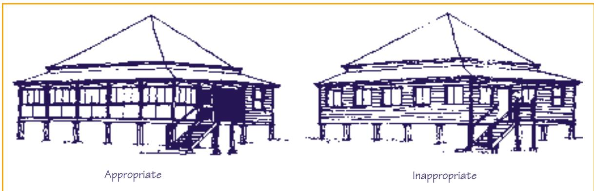
Figure k Appropriate and inappropriate enclosure of verandahs
