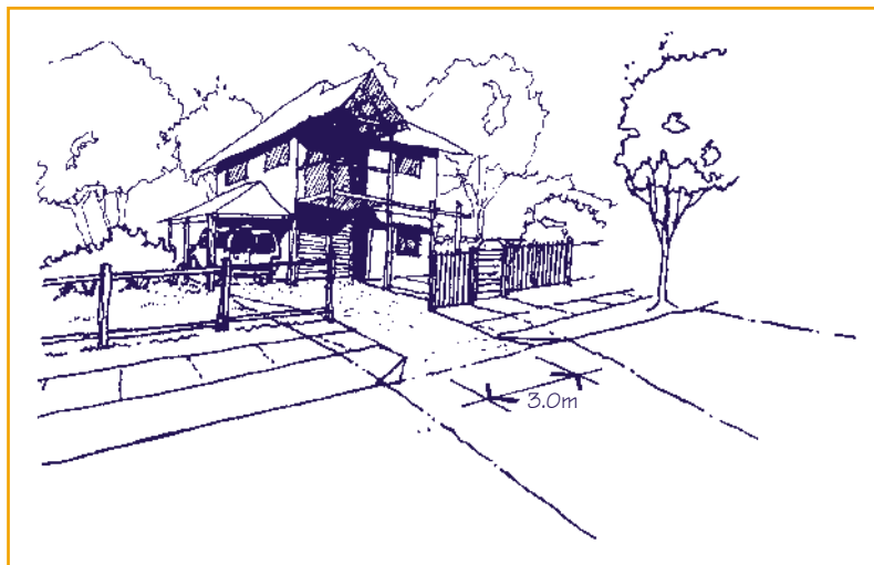
Figure r Double width design, in this case, car accommodation must not dominate the street
