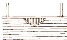
**Cut-outs** Small openings just below the hand rail of a board balustrade, generally infilled with battens and oblong in shape, but sometimes curved like an eyelet.
